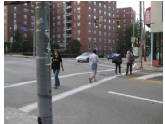
Photo 1 -- A busy intersection, Fifth at Neville, with substantial elderly pedestrian crossings but no ADA ramps at this crossing.
